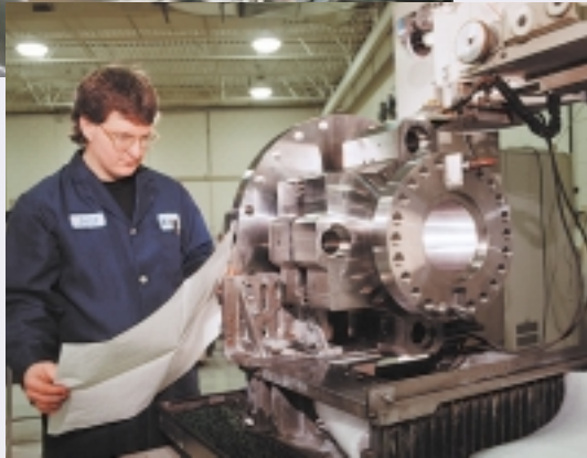
At right, Adron wire EDMed ribs in this 22" stainless steel aerospace component.
